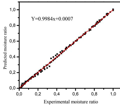
Fig. 7. Comparison of predicted moisture ratio from Midilli-Kucuk model and observed moisture ratio of cherry at different temperatures of drying ( $R^2 = 0.9986$ ).
