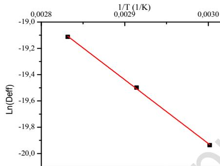
Fig. 3. Arrhenius-type relationship between effective diffusivity and reciprocal absolute temperature.
