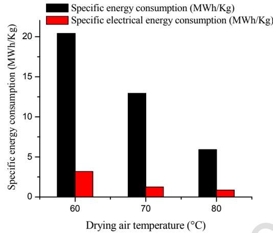
Fig. 5. Specific energy consumption at different drying air temperatures.
